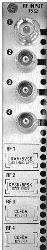
Figure 2-4: Interfaces of the R&S DVM400-B500 RF interface option with the B50, B51, and B52 options
