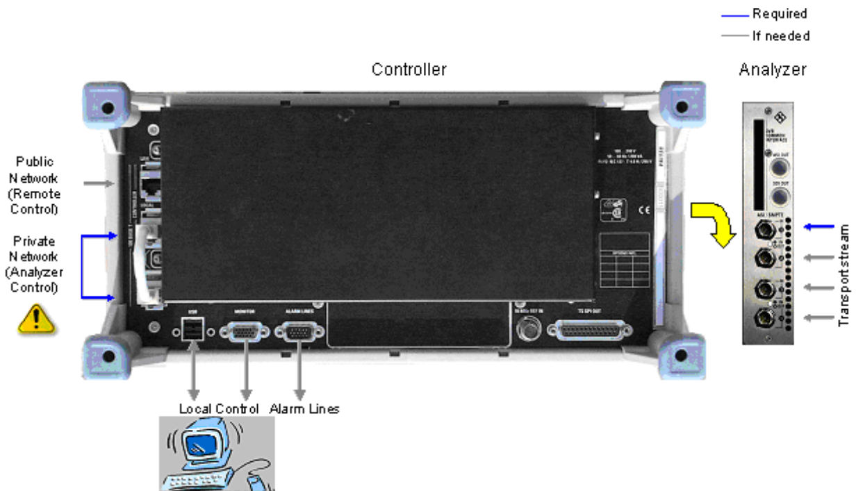
Figure 2-11: Connections of basic configuration of the R&S DVM 400
